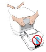
**CAUTION**: Do not use the front end of the Loader as a lift point. Using the Loader to lift the device can damage the baseplate, which is easily bent.
